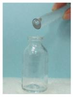
Clean a tube and a glass bottle with clean water. Fill up the tube with sample water and transfer water to the glass bottle.
