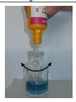
4. Slowly add the Reagent 3 dropwise, swirling to mix after each drop while counting number of drops until a blue end point. The number of drops in this step is designated as "a".
